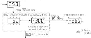
①PV is displayed on operation mode, ②Press MD key, the SV is indicated after "5" is flickering 2 times.
