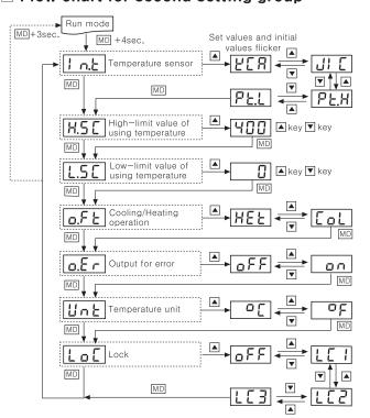
•In operation mode, if press MD key for 4 sec., it enters setting group 2 At the beginning of MD key input, 5 u signal is displayed. And then P signal, the first mode of group 1, is displayed for  $2\sim3$  sec. for the moment of 4 sec past,  $I \cap L$ , the first mode of setting group 2, is displayed. It enters the first mode of group 2 for finishing
