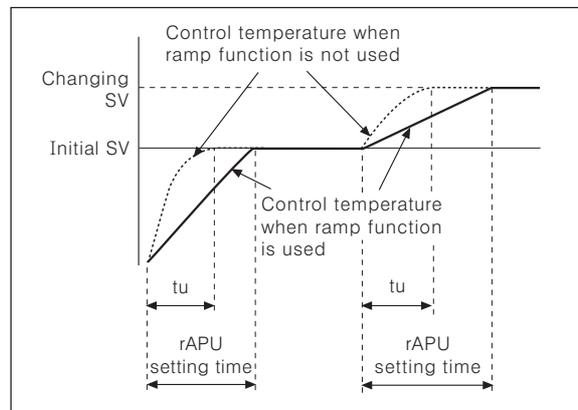
It makes delay rising temperature when change the set value at stable control status or delay the initial rising temperature as like above picture.
