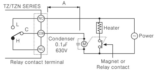
Keep power relay as far away as possible from TZ/TZN series. If wires length of A is short, electromotive force occurred from a coil of magnet switch & power relay may flow in power line of the unit, it may cause malfunction. If wires length of B is short, please connect a mylar condenser 104 (630V) across coil of the power relay "M" to protect electromotive force.
