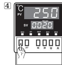
Push **MD** key when the setting is completed. It will stop flickering, then return to **RUN** mode.
