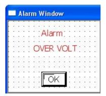
5) When alarm happens, a window will pop out automatically. The operator can take effective measures at once to solve the problem. Press "OK" to close the alarm window.
