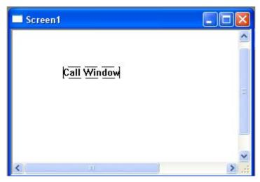
3) Click the property button. Set the relay's type and address in object tab page and set the window No. called in Window tab page. When the middle relay is in the state of ON, the window to be called will popout. When it is OFF, the window will be close. As shown in the following maps.
