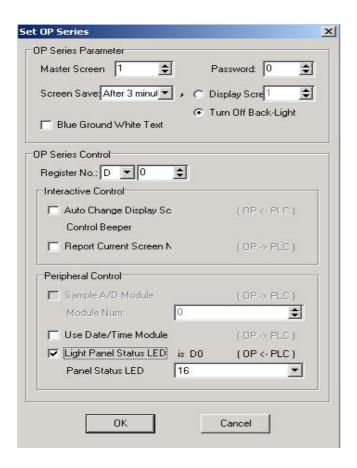
Choose the display function for the status indicate lamp. The 16 button indicate lamps are each controlled by Bit0-Bit10 of D0 register. Its correspond relationship is the following:
