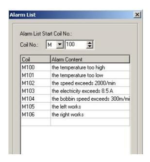
When OP320 works in normal, if M101, M102, M105 are set ON, then the display will auto pop out the alarm screen, and displays like that:
