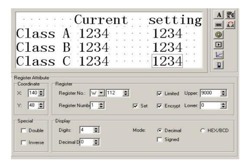
Note: The order of the three data set windows being edited (i.e. mouse's click order) is the same with the order set when operating in practice. If click three data set elements from top to the bottom before saving a project, when running, first set the production of class A, then class B, the last class C.
