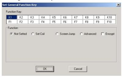
The dialog box displays 20 function keys (K1~K10,F1~F10), here what is displaying is the function's status of display's button [K1] (the program is defaulted). We can see that each function key has 4 functions that can be set. The first three is single select function, which can choose only one function. Encrypt is multi-select function, it can be used with other function keys.
