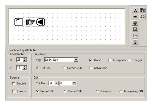
In the function column, select the "SET" button to be the auto mode setting button. Set the coil's define No. to be M10, and set the action mode to be ON. In order to display in brief, cancel the hand display.
