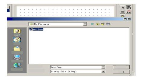
Select the bitmap file which intend to display, then double-click it or click on the open button, there will be a rectangle dashed frame moves with the mouse. Move to the proper position and click the mouse's left key to confirm.
