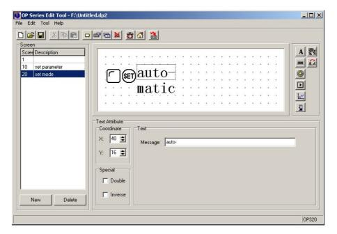
Set the manual button and the manual status indicate lamp with the same method. The address of the indicate lamp is still M10. Choose the display property negative logic. The appointed button is "ENT" button, the button's function is set M10 relay OFF.
