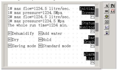
At last, edit the bar curve screen, choose No.30 screen (If it does not exist, create a new one, press key). In the screen description text box, fill in the bar curve.
