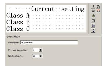
Lay the data display window, click the button, there will be a rectangle dashed frame moves with the mouse, move it to proper position, then click on the left button of mouse to confirm it.
