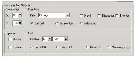
Set water set function key. Press key, in the screen edit area, there will be a rectangle dashed frame moves with the mouse, put it in the proper position. In its property box,
