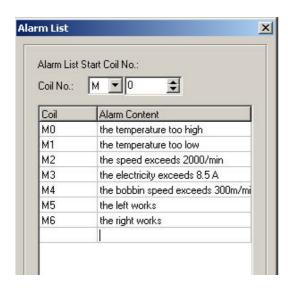
After all the alarm information been input, change the coin's No. to be M100 (example), i.e. it indicates that M100 to M106 individually corresponds with the 7 pieces of alarm information.
