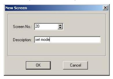
Click [OK] button to confirm. Then there will be the screen's property content displays in the bottom of the interface. Set the previous screen No. to be 0 and the next screens No. to be 10. In the running status, press " $\land$ " to directly enter the menu screen, press " $\lor$ " key to enter parameter setting screen.
