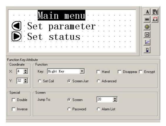
In the main menu screen, add an alarm screen jump key. When click this key, you can jump to the alarm list screen, refer to the alarm information.
