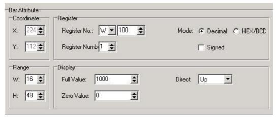
Place bar graph, real time display No.1 valve's flow. Press key, in the screen edit area, there will be a rectangle dashed frame moves with the mouse. Place it in the proper position. In the bar graph property box, set register's ID W101. The full rated value is 1000, set width 26, set height 80. The bar graph will real time display No.1 valve's flow.
