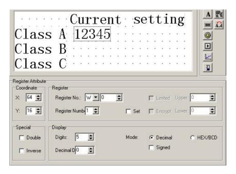
Display "12345" these five numbers inside the dashed frame, that means that this element is a register display window or register set window whose length is five bits.
