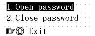
Select 1, execute the operation of opening password; select 2, make the system be in the status of password closing. Click on the button, return back to the monitor status.
