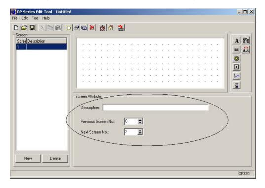
First, enter the edit status of the system's initial screen (If default it will be the No.1 screen). In the bottom of the screen is the current screen's (No.1 screen) property, each screen has the property, include three items of the content.
