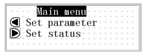
The No.1 screen is a menu screen, Shift directly to the sub screen via the function key. Press "<" key to directly enter the parameter set screen (No.10 screen).
