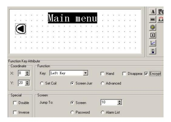
After set the function key, place text "set parameter" to the right of the button graph to prompt the operator. Click "<" key to enter parameter set screen directly.
