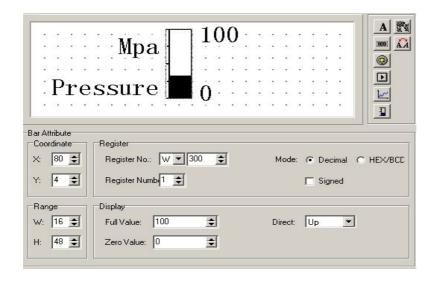
This bar monitors the value in D300. When the bar displays in the full scale, it indicates that the value in D100 is 100; when the bar displays in 50% scale, it indicates that the value in D300 is 50.
