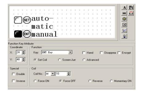
Set two circle indicate lamps, positive logic. Each one's address is M20 and M21, monitor the motor's work states. When the indicate lamp in the left lights, it means the motor is rolling ahead, when the indicate lamp in the right lights, it means the motor is rolling back.
