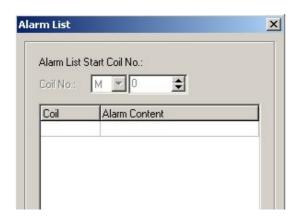
As there is no input content, the alarm list's content is vacant. First, move the cursor to the 《alarm content》 column, then write the alarm information "the temperature too high" into it. After confirming by entering the screen will display:
