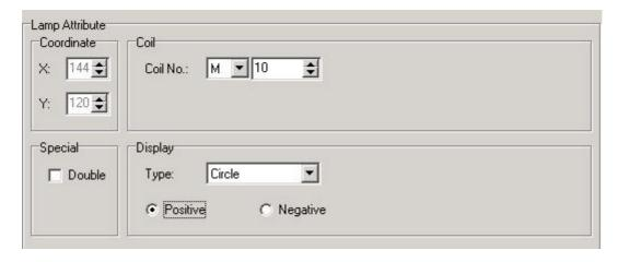
Place "No.1 storage hollow" indicate lamp, press key, there will be a rectangle dashed frame moves with the mouse, place it in the proper position. In the indicate lamp property dialog box, modify the coil's ID to be M11, the indicate lamp will display the status of No.1 storage (M11). When the indicate lamp change from hollow to solid (positive logic), it means that No.1 storage is hollow.
