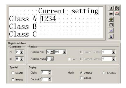
Set the current values display window of Class B and Class C with the same method. The addresses of registers are D101 and D102 respectively, other properties are the same as before.
