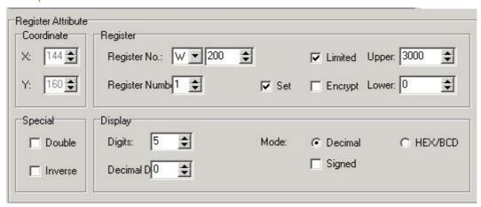
Place the data window for No.2 valve's max flow setting. Press key, there will be a rectangle dashed frame moves with the mouse. Place it in the proper position. In the data register property dialog box, set the register's ID as W201. Choose the set function, choose the max and mini limitation, set the max limitation as 30000, the mini limitation as 0. The data window will set No.2 valve's max flow.
