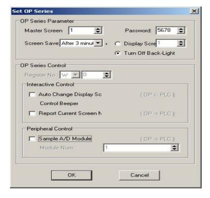
Input the password or modify the original password, e.g. input password "5678", then press "OK" button, the password is confirmed.
