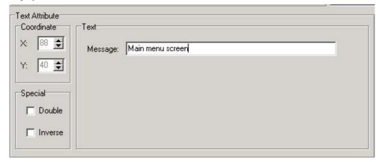
Choose the text "status", choose inverse phase property for the text property frame. The text bunch "status" will display in the format of inverse phase. Display the text bunch "monitor", "parameter", "setting", "bar graph", "curve", "alarm", "list" etc. in the format of inverse phase with the same method.
