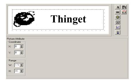
Note: it can display a bitmap with 192×64 pixels at most. The extra part will be removed automatically.
