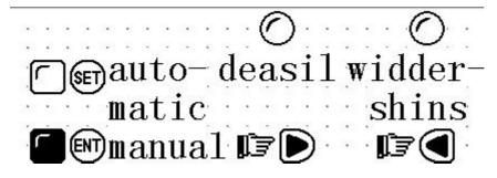
Now, the device is in the manual mode, click the "SET" button to set the device to be automatic mode, i.e. M10 of the PLC is set ON.
