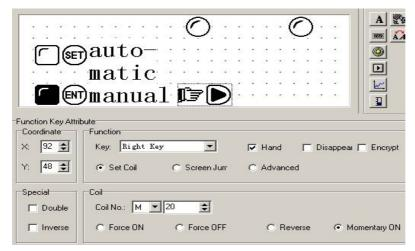
Click the button to place the function key, select "<" button, its address corresponds with M21, its function is momentary set M21 relay to be ON, and keep the hand graph. It indicates that when click on the "<" button, M21 of PLC is set to be ON, and the motor begins to run back. (PLC program, use M21 to trigger Y0); when release the ">", M21 recovers to the OFF status, and the motor stops running back.. At last place the text "run ahead" and "run back" to be the clue.
