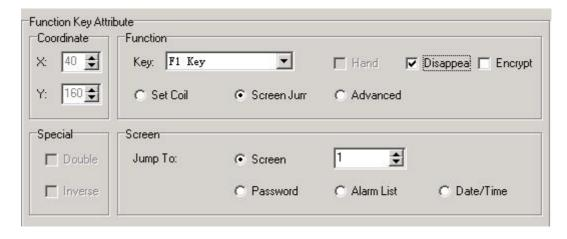
Place the function key F2, press key, place it in the proper position. In the property dialog box, choose the key value as F2, set it concealed, choose screen jump function, the screen will jump to No.20 screen.
