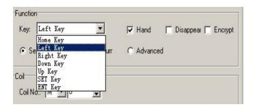
Considering to be brief, you can cancel hand display, then in the screen there will be only a button. After this set the function to be screen jump, here underside the screen set the jump screen's ID number. Set the target screen's ID number to be 10, i.e. the tenth screen is the parameter set screen.
