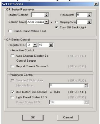
Choose "Use Data/Time Module", set the control register's No. you use. E.g. set it to be D46, then the clock's data will be placed into three groups of registers which start with D46. D46 will store of year and month, D47 will store data of date and hour, D48 will store data of minute and second.
