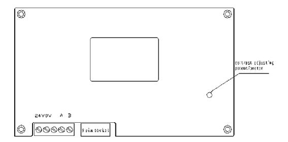
On the left of European-style terminal table is the exterior-connect DC power terminal, on the right is the connection interface of RS485 communication port. RS232 and RS485 communication ports are placed in the DB9 socket. When downloading the screen data, connect the 9 pin communication port of OP320 and that of the personal computer with communication cable OP-SYS-CAB. When communicating with PLC, make sure the communication port's connect format according to the PLC type.
