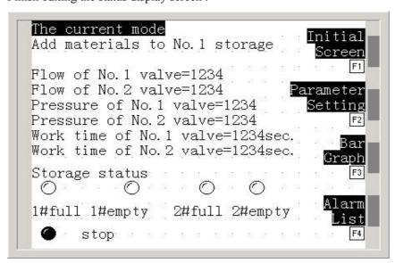
Next, edit the parameter to set the screen, choose No.20 screen (if it does not exist, then create a new one, press key). In the screen description box, fill in the parameter setting.
