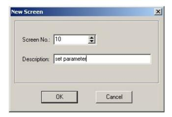
Click [OK] button to confirm. After that, there will be the content of screen attribute in the right bottom of the screen. Set the "Previous Screen No." to be 0, set the "Next screen No." to be 20. Then in the normal display status (not in the status of data setting), click " $\wedge$ " key to directly enter the main menu screen, click " $\vee$ " key to directly enter the state setting screen
