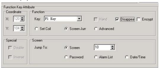
Place function key F2. Press key to place the button at the proper position. In the property frame, choose the key's value to be F2. Set it concealed. Set screen jump function, the screen will jump to No.20 screen.
