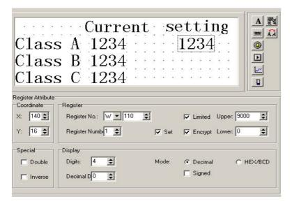
Set the other properties in turn: register No. = D110; Register number = 1; Data digits = 4; Decimal number = 0; display in decimal system. Set the production set window of Class B and Class C with the same method. The set value of Class B corresponds with D111, and the setting value of Class C corresponds with D112.
