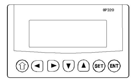
All the 7 keys can be defined to have special function. Such as bit set, bit reset and screen jumping etc. It can only execute the basic function if it has not been defined as special function. The basic functions include set register values, reset the initial screen, jump to the between the former or next screen.
