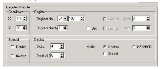
Place the display window, display the flow of No.2 valve. Press key and there will be a rectangle dashed frame moves with the mouse in the screen edit area. Place it at the proper position and click the mouse's left key. In the data register property dialog box, modify the register's No. to be W101, modify the display digit to be 4, the data window will display the flow of No.2 valve.
